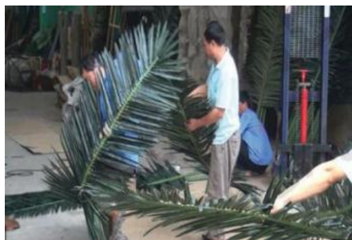
第三步：把叶片往背面弯成C型。 Step3: Bend the leaves back into a C shape
