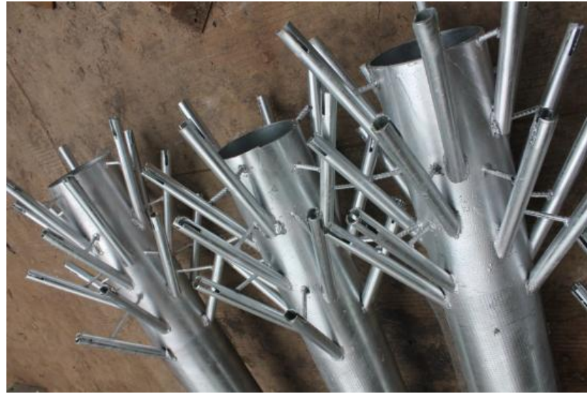
蒲葵树钢结构 Fan Palm Tree Interior Structure
